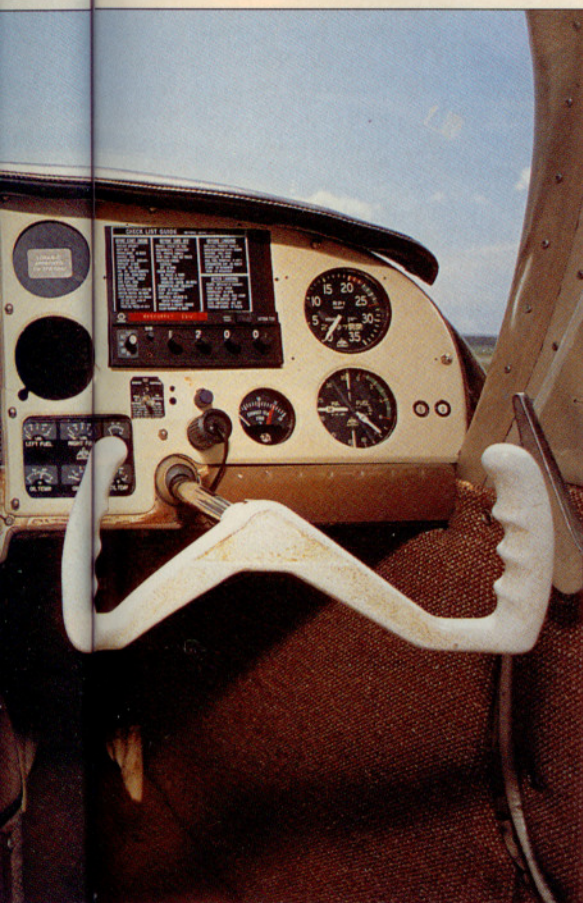
The old-style instrument panel is nonstandard and none too large: The flap handle (right, in above photo) is attached to the hydraulic pump; the gear handle is to the left.
